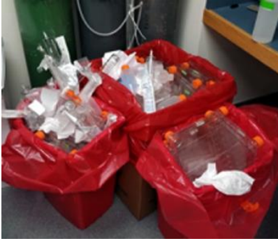
The use of flask culture for the production of exosomes can generate a large amount of waste. This is an example of the number of flasks used to generate 1 \times 10^9 cells.
