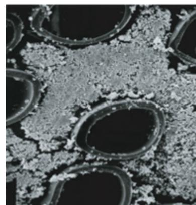
**Figure 24: Cross section of hollow fibers**
