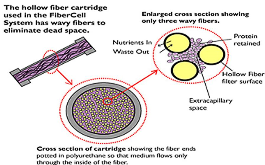
**Figure 7: Diagram of a hollow fiber bioreactor**
