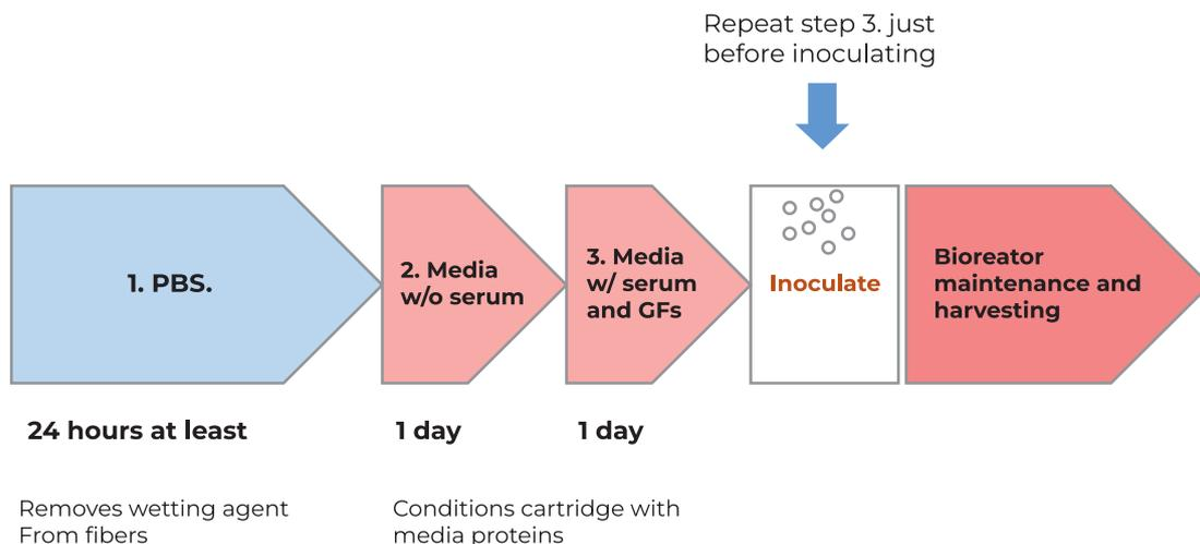
Figure 15: Block diagram of steps involved in setting up and seeding a cartridge.
