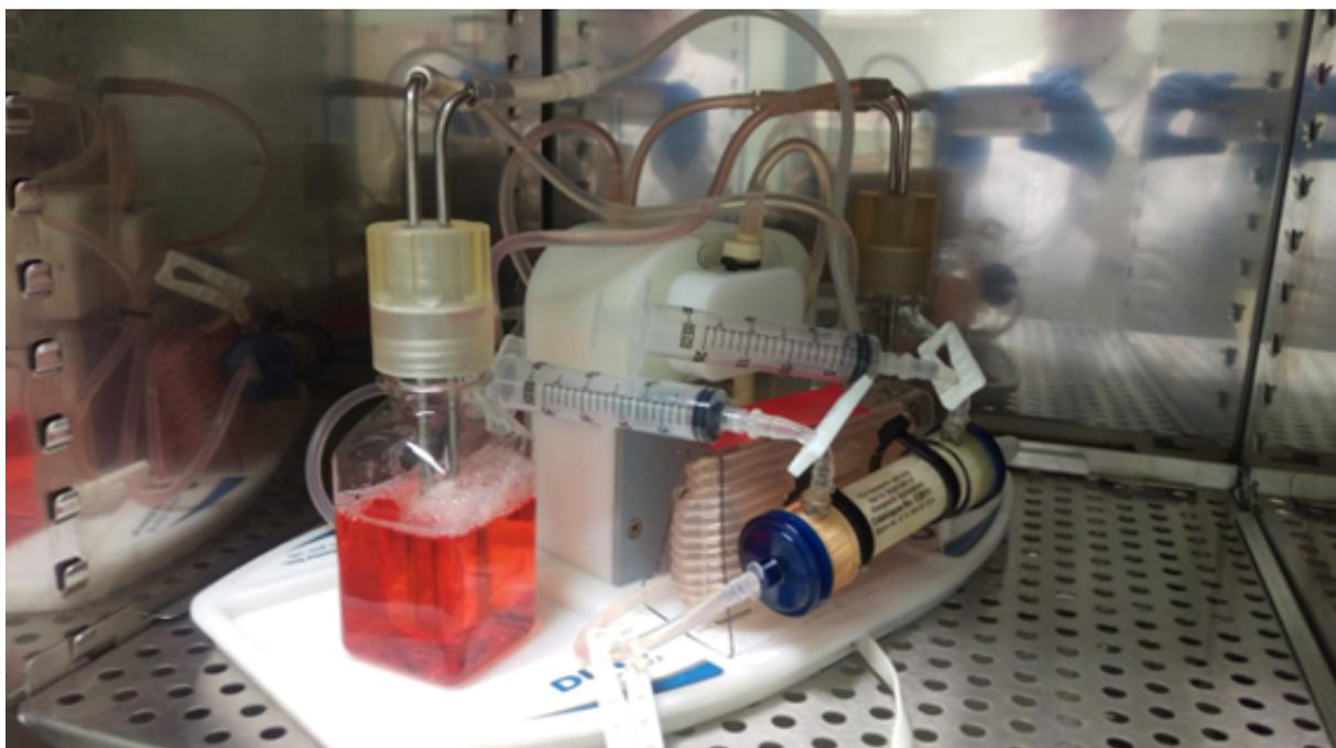
**Figure 1: FiberCell Systems' 3D Hollow Fiber Bioreactor with Duet Pump in an Incubator.**
