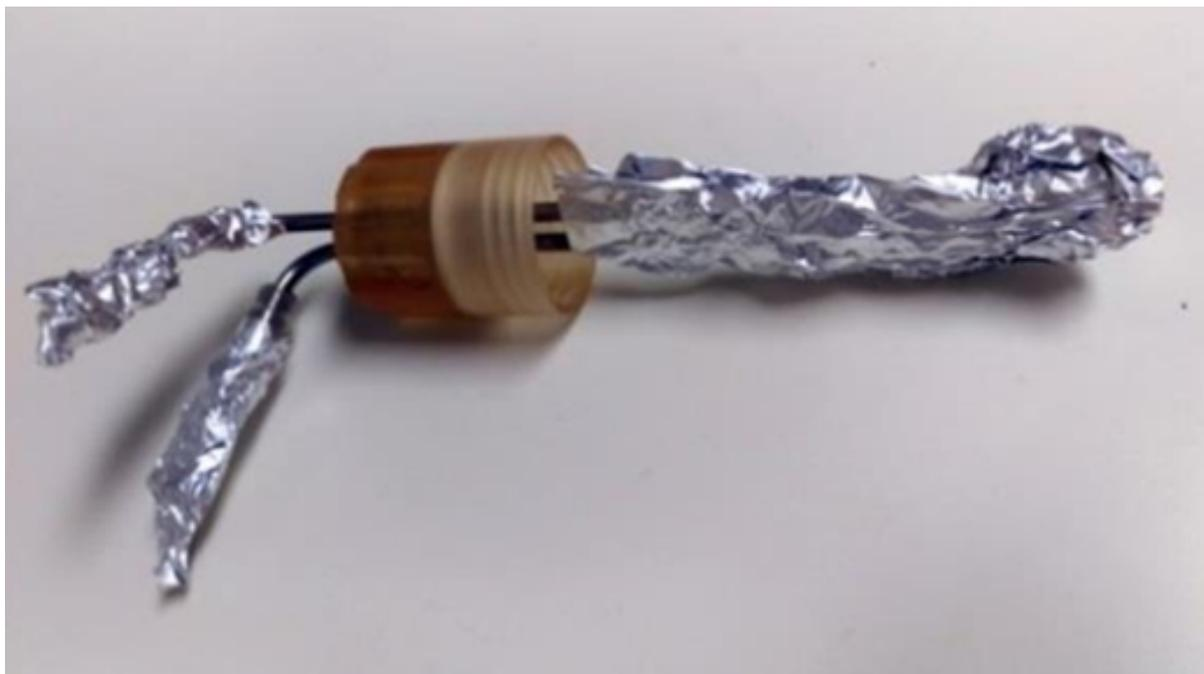
**Figure 13: Aluminum foil protects the exposed parts of the reservoir cap. Once placed in autoclave bag the reservoir is ready to be autoclaved. Place the reservoir cap tubing on the hose barbs of the cap prior to autoclaving.**
