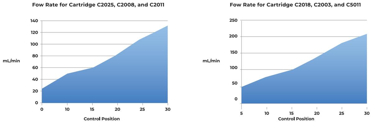
**Figure 20: Duet flow rates vs. control knob position.**
