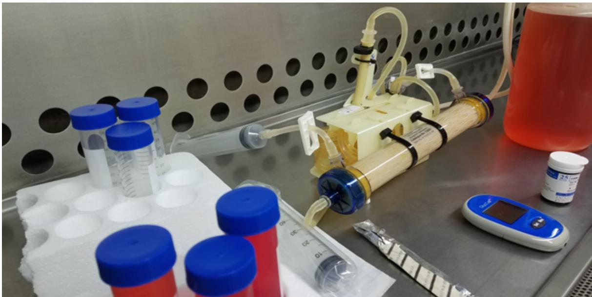
Figure 3: FiberCell Systems' 3D Bioreactor (C2018 Large Cartridge) with Harvests.
