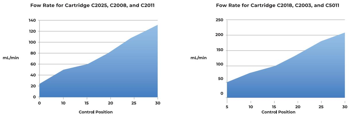
**Figure 35: Duet flow rates vs. control knob position.**
