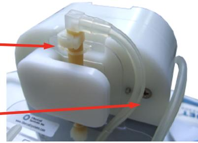
**Figure 30: Pump tubing**
