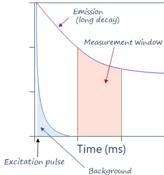
Figure 2: Illustration of TRF principle.
